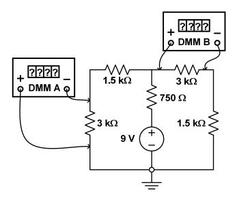
(a) (12.5 points) Find the DMM readings if both of them are set to measure voltage, and indicate the units. (Note: Pay attention to the polarities of each DMM!)
