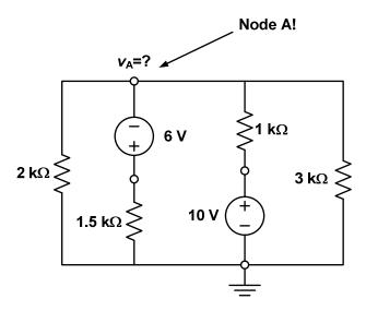
4. (25 Points) In the circuit shown, find the current  $i_x$  that flows through the 3 k $\Omega$  resistor. Please show your work step by step.
