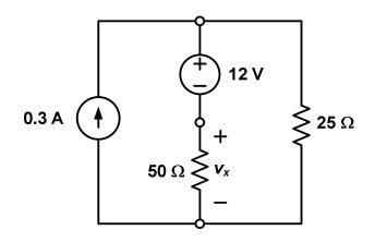
4. (25 Points) In the circuit shown, find the power of each voltage source. Indicate the type of each power (i.e., supplied or absorbed). Please show your work step by step.
