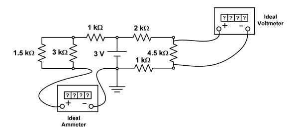
(a) (12.5 points) Find the two DMM readings. Please indicate the appropriate units. (*Note:* Pay attention to the polarities of each DMM!)
