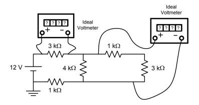
(a) (12.5 points) Find the DMM readings if both of them are set to measure voltage, and indicate the units. (Note: Pay attention to the polarities of each DMM!)
