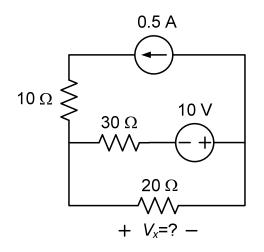
4. (25 Points) In the circuit shown, first, find the node voltages v<sub>a</sub>, v<sub>b</sub>, and v<sub>c</sub>. Then, use these node voltage values to determine the power of each element. Indicate the type of each power value (i.e., absorbed or supplied). Please show your work step by step. Don't forget to calculate the power values!
