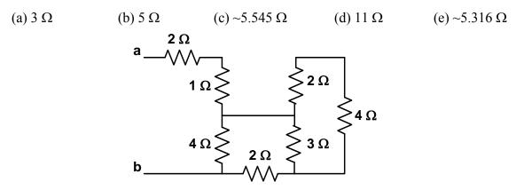
**P-40. Equivalent resistance.** For the resistive network shown below, between which two terminals the equivalent resistance will be the largest in value?
