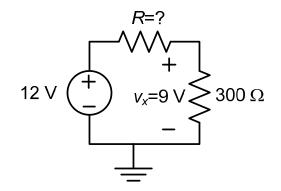
**P-6. Kirchhoff's and Ohm's laws. (Voltage divider principle.)** What is the voltage v in the circuit shown below?
