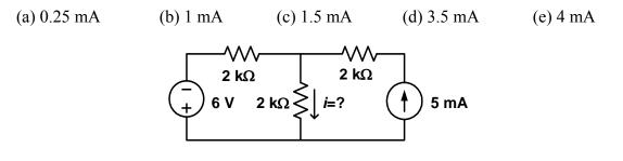
**P-49.** Superposition principle. In the circuit shown, what is the power dissipated by the  $2 \Omega$  resistor?
