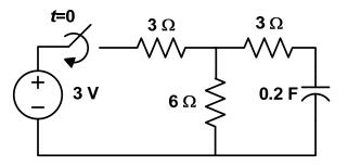
**P-84. Time constant of a first-order circuit.** What is the time constant of the first-order *RL* circuit shown after the switch is closed at *t*=0?
