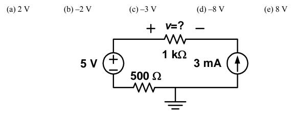
**P-46.** Node voltage. For the circuit shown below, what is the node voltage  $v_A$ ?
