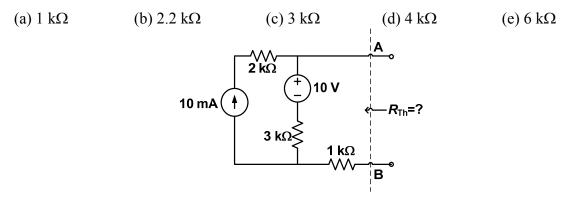
**P-64. Norton resistance.** For the circuit shown, what is the Norton resistance seen between the terminals "x" and "y"?
