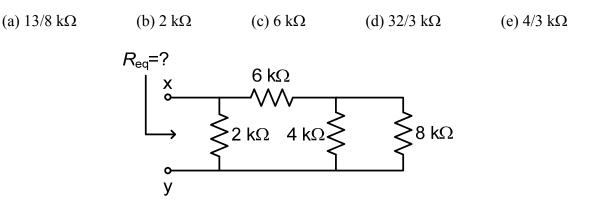
**P-39. Equivalent resistor.** In the circuit shown below, what is the equivalent resistance seen between terminals "a" and "b"?
