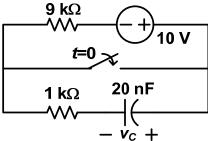
**P-88.** A first-order circuit with two capacitors. In the following circuit shown, the switch closes at t=0, after being open for a long time. Approximately how long will it take for the capacitor voltage  $v_c$  to reach 99% of its final value?
