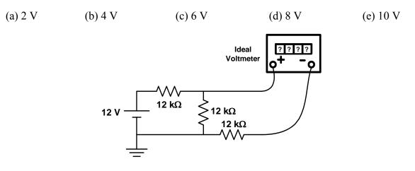
**P-28. Voltmeter and ammeter measurements.** For the dc circuit shown below, what are the readings of the voltmeter and the ammeter? (Assume ideal meters.)
