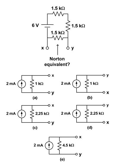
**P-61. Norton equivalent circuit.** For the circuit shown, what is the Norton current and the Norton resistance seen between the terminals "a" and "b"?
