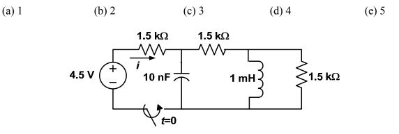
**P-95. First-order switching** *RC* circuit. For the first-order *RC* circuit shown below, the switch is closed at t = 0, after being open for a long time. Which one of the following voltage expressions represents the voltage  $v_c(t)$  for  $t \ge 0$ ?
