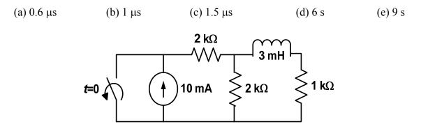
**P-83. Time constant of a first-order circuit.** What is the time constant of the first-order *RC* circuit shown below after the switch is closed at *t*=0?
