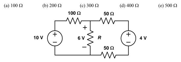
**P-53. Kirchhoff's and Ohm's laws.** For the circuit shown below, what is the total power supplied by the two voltage sources?
