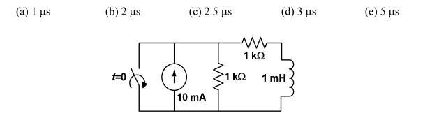
**P-97. Second-order switching circuit.** In the second-order circuit shown below, the switch closes at t = 0, after being open for a long time. Which one of the following is the value of the voltage  $v_x$  right after the switch closes (i.e.,  $v_x(0^+) = ?$ )?
