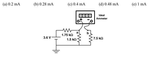
**P-26.** Ammeter reading. To measure the current through the 7.5 k $\Omega$  resistor of the circuit in Problem 12, a student makes a mistake and connects the ammeter in parallel with that resistor as shown below. What will be the reading of the ammeter in the circuit below? (Assume ideal ammeter.)
