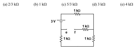
**P-68.** Power delivered to the load. In the circuit of the Problem 67, if a load resistance of value  $R_L \cong 1.67 \text{ k}\Omega$  is connected between "e" and "f" terminals, what power is delivered to  $R_L$ ?
