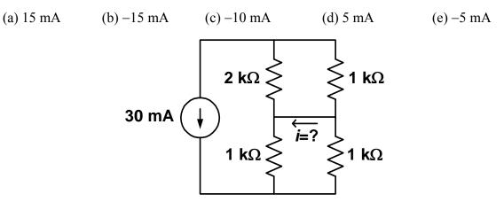
**P-42. Current divider principle.** For the circuit shown below, what is the current  $i_x$ ?
