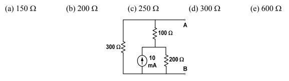
**P-58. Thévenin equivalent circuit.** For the circuit shown, what is the Thévenin voltage and the Thévenin resistance seen between the terminals "a" and "b"?
