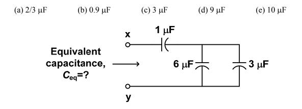
**P-74. Equivalent capacitance.** In the circuit shown below, what is the equivalent capacitance  $C_{eq}$  seen between the "x" and "y" terminals of the voltage source?
