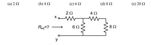
**P-38. Equivalent resistance.** For the resistive network shown below, what is the equivalent resistance  $R_{eq}$  seen between terminals "x" and "y"?
