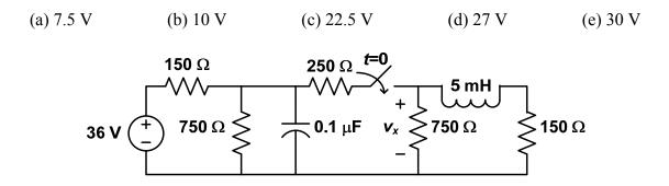
**P-98. Second-order switching circuit.** In the second-order switching circuit shown below, the switch opens at t = 0, after being closed for a long time. What is the value of the capacitor current  $i_c$  right after the switch opens? (That is, what is  $i_c(0^+)$ ?)
