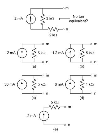
**P-60. Norton equivalent circuit.** Which one of the following is the Norton equivalent of the circuit shown at the top below?
