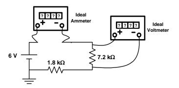
**P-29. Voltmeter and ammeter measurements.** The ammeter and the voltmeter in the previous circuit are switched as shown below. What will be their new readings? (Again, assume both voltmeter and ammeter to be ideal.)
