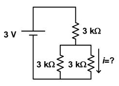
**P-18. Current divider principle.** For the dc circuit shown, what is the current *i* flowing through the 3 k $\Omega$  resistor?
