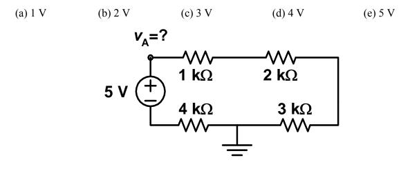
**P-47. Node voltage.** For the circuit shown, what is the value of the node voltage  $v_x$ ?
