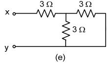
**P-37. Equivalent resistance.** For the resistive network shown below, what is the equivalent resistance  $R_{eq}$  seen between terminals "x" and "y"?
