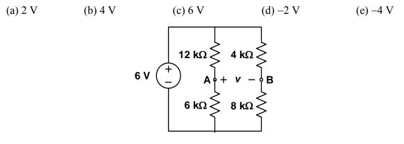
**P-34. Current divider principle.** For the circuit shown below, which one of the following relationships is *not* correct?
