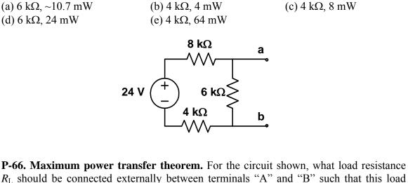
**P-66.** Maximum power transfer theorem. For the circuit shown, what load resistance  $R_L$  should be connected externally between terminals "A" and "B" such that this load resistance will receive maximum power possible from the rest of the circuit and what is the maximum power absorbed by this load?
