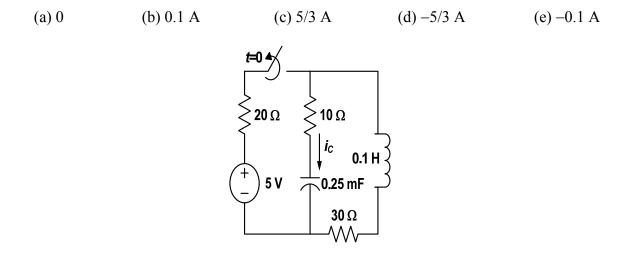
**P-99.** Natural response of a second-order circuit. For the second-order circuit of Problem 98 shown above, right after the switch opens at t = 0, what is the <u>total</u> energy stored in the circuit at  $t = 0^+$ ?
