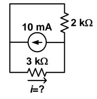
**P-13. Kirchhoff's laws and power.** For the circuit shown, which box elements dissipate power?
