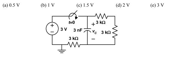
**P-86. Time constant of a first-order circuit.** In Problem 85, what is the time constant of the circuit after the switch closes at t=0?
