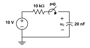
**P-78. First-order capacitive circuit.** In the first-order capacitive circuit shown below, the switch closes at t=0. If the capacitor voltage is initially 10 V, which one of the following is the correct mathematical expression for  $v_R(t)$  valid for t > 0?
