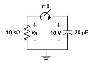
**P-79. First-order capacitive circuit.** In the circuit shown below, the switch closes at t = 0, after being open for a long time. Which one of the following expressions represent the capacitor voltage  $v_c(t)$  for  $t \ge 0$ ?
