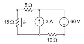
5. (20 Points) In the electric circuit shown, determine the value of the current  $i_y$ . Show your work step by step.
