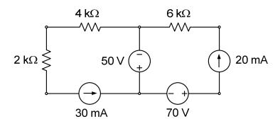
2. (20 Points) Consider the electric circuit shown. Determine the values of each node voltage  $v_a$ ,  $v_b$ ,  $v_c$ , and  $v_g$ . Show your work step by step including justifications. Box your answers with appropriate units.
