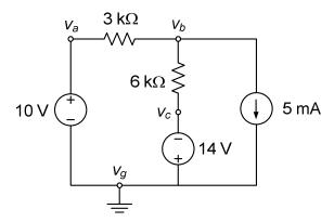
3. (20 Points) Consider the electric circuit shown. Determine the voltage  $v_a$  across the 3 k $\Omega$  resistor on the right-hand-side as indicated. Please provide your work step by step with justifications. Box your answer.
