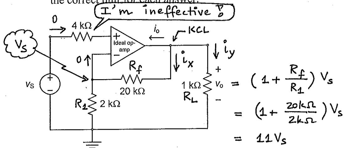
$$(a) \quad v_s = \frac{1}{2} \text{ V} \rightarrow v_o = \frac{11}{2} = \boxed{5.5 \text{ V}}$$
