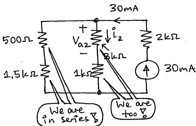
$$\text{CDP} \rightarrow i_2 = \frac{2\text{k}\Omega}{(2+4)\text{k}\Omega} (30\text{mA}) \\ = 10\text{mA}$$
