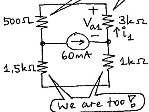
$$\text{CDP} \rightarrow i_1 = \frac{2.5\text{k}\Omega}{(2.5+3.5)\text{k}\Omega} (60\text{mA}) \\ = 25\text{mA}$$
