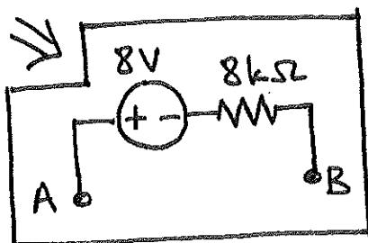
Problem 3 (20 POINTS). Consider the circuit shown below. Determine the value of the unknown resistance  $R$  such that it will receive maximum power from the circuit. What is the maximum power received by the  $R$  resistor you have chosen? Show your work step by step. Note that you need to provide two answers for this problem.
