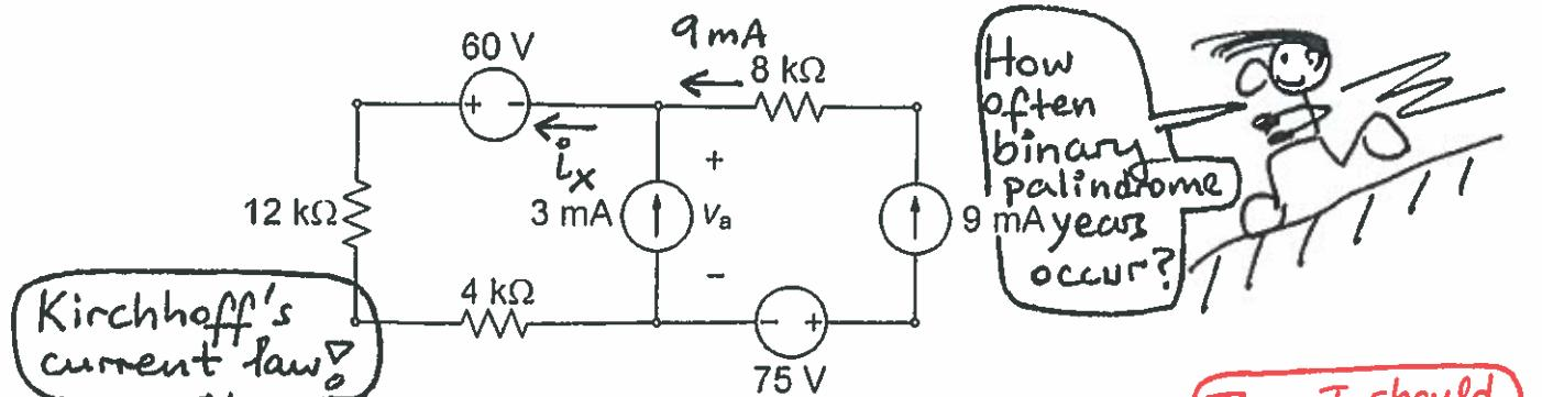
$$KCL \rightarrow i_x = 3 \text{ mA} + 9 \text{ mA} = 12 \text{ mA}$$
