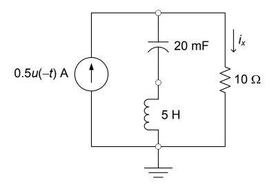
(a) (15 points) Solve for the roots ( $s_1$  and  $s_2$ ) of the characteristic equation of the above circuit for  $t \ge 0$ .
