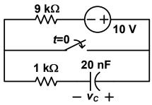
**P-88.** A first-order circuit with two capacitors. In the following circuit shown, the switch closes at t=0, after being open for a long time. Approximately how long will it take for the capacitor voltage  $v_c$  to reach 99% of its final value?
