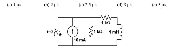
**P-97. Second-order switching circuit.** In the second-order circuit shown below, the switch closes at t = 0, after being open for a long time. Which one of the following is the value of the voltage  $v_x$  right after the switch closes (i.e.,  $v_x(0^+) = ?$ )?
