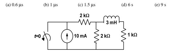
**P-83. Time constant of a first-order circuit.** What is the time constant of the first-order *RC* circuit shown below after the switch is closed at t=0?
