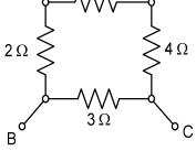
**P-41. Current divider principle.** For the circuit shown below, what is the current *i*?
