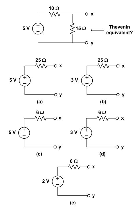
**P-55. Thévenin equivalent circuit.** Which one of the following is the Thévenin equivalent circuit between the "x" and "y" terminals of the circuit shown below?
