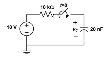
**P-78. First-order capacitive circuit.** In the first-order capacitive circuit shown below, the switch closes at t=0. If the capacitor voltage is initially 10 V, which one of the following is the correct mathematical expression for  $v_R(t)$  valid for t > 0?
