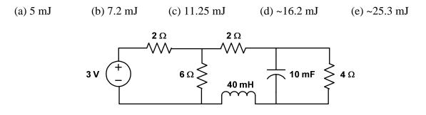
**P-92. Energy stored in an inductor at steady state.** For the second-order circuit shown below, what is the energy stored in the 5-mH inductor at steady state?
