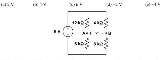
**P-34. Current divider principle.** For the circuit shown below, which one of the following relationships is *not* correct?
