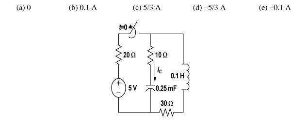
**P-99.** Natural response of a second-order circuit. For the second-order circuit of Problem 98 shown above, right after the switch opens at t = 0, what is the <u>total</u> energy stored in the circuit at  $t = 0^+$ ?
