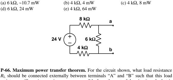
$R_{\rm L}$  should be connected externally between terminals "A" and "B" such that this load resistance will receive maximum power possible from the rest of the circuit and what is the maximum power absorbed by this load?
