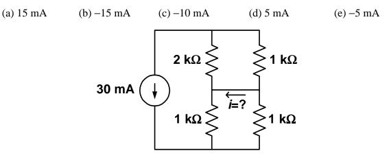
**P-42. Current divider principle.** For the circuit shown below, what is the current  $i_x$ ?
