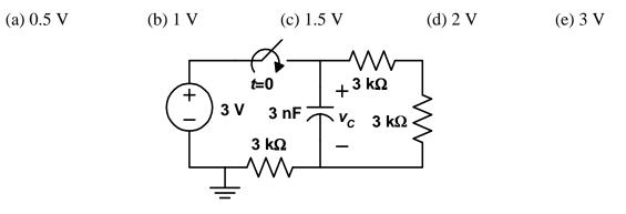
**P-86. Time constant of a first-order circuit.** In Problem 85, what is the time constant of the circuit after the switch closes at t=0?
