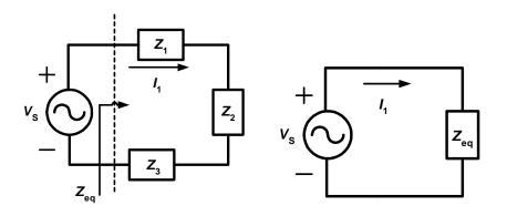
**4.h. Thevenin impedance.** For the phasor-domain circuit shown, given the three impedance values to be  $Z_1 = 50 \Omega$ ,  $Z_2 = j50 \Omega$ ,  $Z_3 = -j50 \Omega$ ,  $Z_{Th} = Z_3 + \frac{Z_1 Z_2}{Z_1 + Z_2} = ?$
