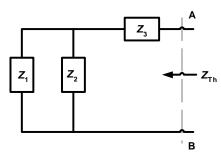
**4.i. KVL and Ohm's law.** In the phasor-domain circuit shown below, given  $Z_1 = (300 + j300)\Omega$ ,  $Z_2 = 300\sqrt{2}e^{-j\pi/4}\Omega$ ,  $I_x = 0.04e^{j\pi/3}A$ ,  $V_x = (Z_1 + Z_2)I_x = ?$
