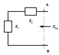
**4.d. Equivalent impedance of a series** *RLC* **circuit.** In the series *RLC* circuit shown, the element values are given by  $R = 4 \Omega$ , L = 5 mH, and C = 1.25 mF respectively. Find the equivalent impedance of this circuit at three different frequencies:  $\omega_1 = 200 \text{ rad/s}$ ,  $\omega_2 = 400 \text{ rad/s}$ , and  $\omega_3 = 1,200 \text{ rad/s}$ .
