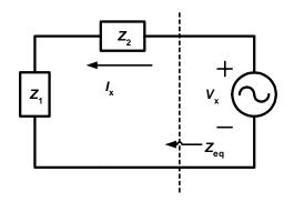
**4.j. KCL and Ohm's law (optional).** In the following phasor-domain circuit shown,  $Y_1 = 0.02e^{-j\pi/2}$  S,  $Y_2 = 0.01\sqrt{3}e^{j\pi/3}$  S,  $V_y = e^{j60^\circ}$  V,  $I_y = (Y_1 + Y_2)V_y = ?$
