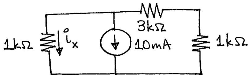
(8) For the circuit shown, find the power of each source and provide your answers based on passive convention.
