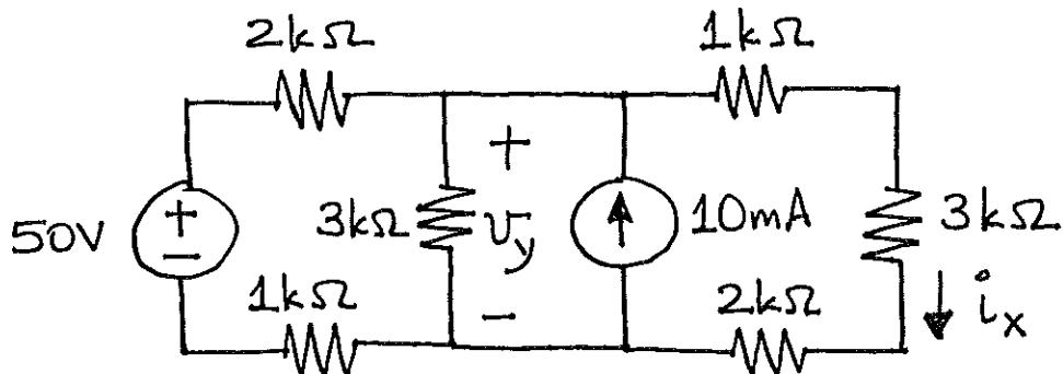
(10) For the circuit shown, find the power of each element. Also, verify conservation of energy principle.
