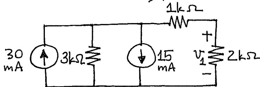
(14) For the circuit shown, find the current through the 1 kΩ resistor.
