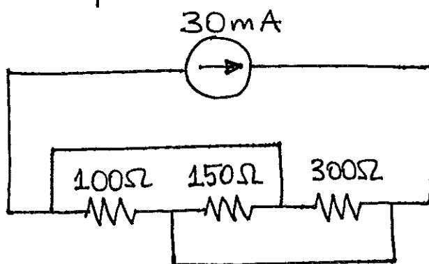
(12) For the circuit shown, find the power of each element and verify conservation of energy principle.
