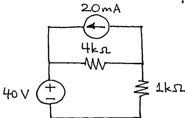
(11) For the circuit shown, find the value and direction of the current of each resistor.
