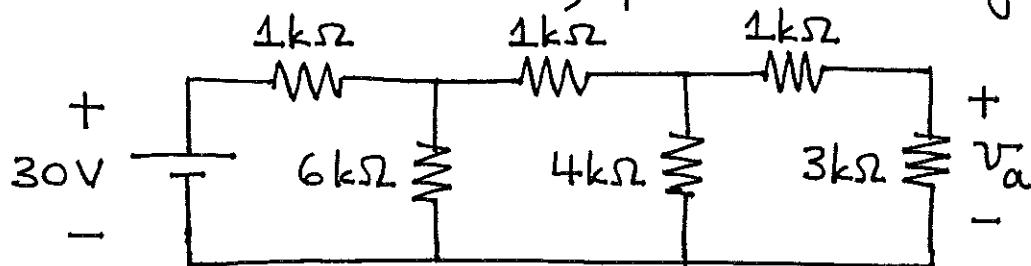
(16) For the circuit shown, find the current through each resistor including their directions.
