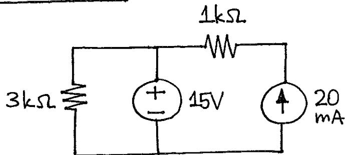
(13) In the circuit shown, find the value of voltage  $v_1$ .
