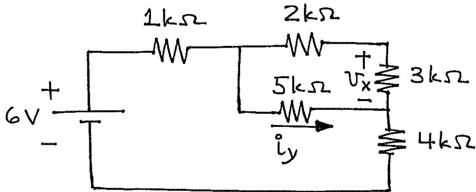
(6) For the circuit shown, find the currents  $i_1, i_2, i_3$  and  $i_4$ .
