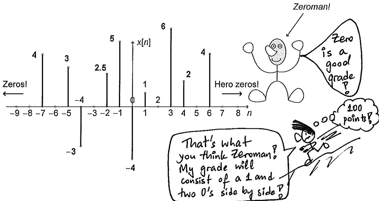
(a) (10 points) Find and sketch the signal  $v[n] = x[1-3n]$ . (Do the time shifting before the time scaling.)
