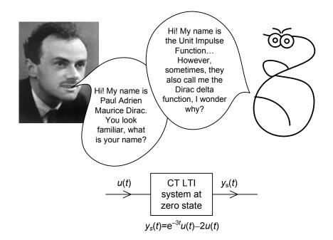
(3) (15 mins., <u>Total:</u> 20 points) **CT LTI system.** The unit-step response  $y_s(t)$  of a continuous-time (CT) linear time-invariant (LTI) system is given as shown.
