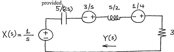
(b)(10) Using part (a) circuit, obtain Y(s) and perform inverse Laplace on it to obtain y(t) for t > 0.
