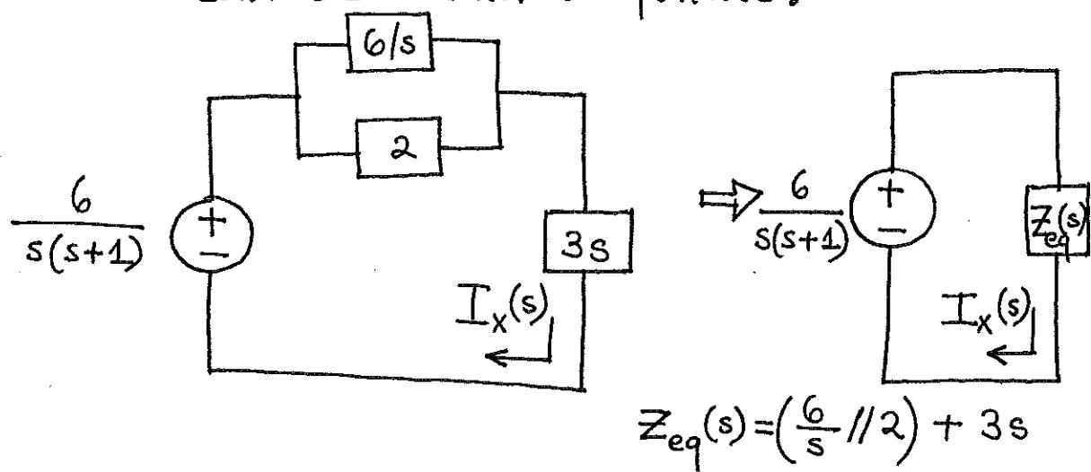
(b) (15 points) Using the circuit drawn in part (a), find the complete simplified mathematical expression for the current  $i_x(t)$  for  $t \geq 0$ .
