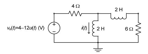
(a) (10 points) Draw the complete unilateral Laplace domain equivalent circuit with all the pertinent values included. Show how you obtain the initial conditions and how you model them in your equivalent circuit.
