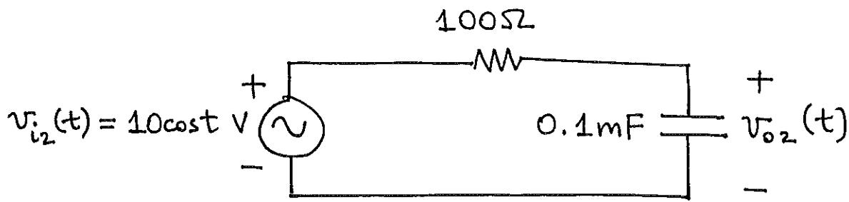
Using the phasor-domain circuit, we find  $V_{o2}(t)$  to be
