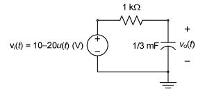
(8) (10 points) **Transfer function and impulse response.** Find the transfer function and the impulse response of the electric circuit shown.
