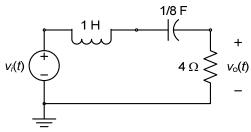
(9) (10 points) Application of Laplace transform to electric circuits. For the electric circuit shown, use Laplace transform to find the output voltage signal  $v_o(t)$  for  $t \ge 0$ .
