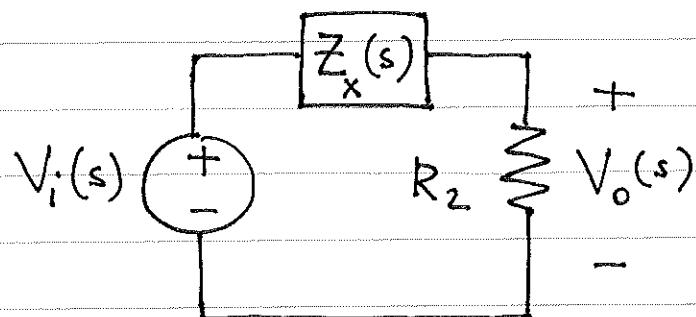
$$V_o(s) = \frac{R_2}{\frac{sR_1L}{sL + R_1} + R_2} V_i(s)$$
