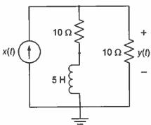
$x(t) = u(t) \rightarrow y(t) = \left[y(0^{\dagger}) e^{-t/\tau} + y(\infty) \left(1 - e^{-t/\tau}\right)\right] u(t)$   $y(0^{\dagger}) = 10 \times 1 = 10 \text{ V} \text{ since } \begin{cases} 1 & \text{acts like open circuit} \end{cases}$   $y(\infty) = 10 \times \frac{1}{2} = 5 \text{ V} \text{ since } \begin{cases} 1 & \text{acts like short circuit} \end{cases}$   $T = \frac{L}{R_T} = \frac{5H}{20\Omega} = \frac{1}{4} \text{ s}$
