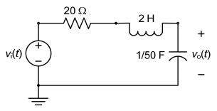
(9)(10 points) Application of Laplace transform to electric circuits. For the electric circuit shown, use Laplace transform to find the current signal  $i_o(t)$  for  $t \ge 0$ .
