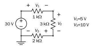
4. Suppose in the circuit below that the currents are found to be  $I_1 = 7.5$  mA and  $I_3 = 2.5$  mA. Determine the value of  $I_2$ .
