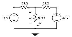
2. (25 points) In the circuit shown, find the values of  $v_x$  and  $i_x$  using the superposition principle. (<u>Hint:</u> Use the results of Problem 1.) Box your answers.
