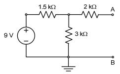
4. (25 points) In the circuit shown, find the value of *R* that will maximize power delivered to the 3 k $\Omega$  resistor. What is the maximum power delivered to the 3 k $\Omega$ ?
