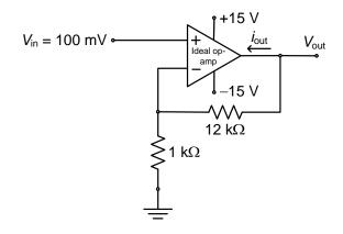
(3) (40 points) In the op amp circuit shown, find  $V_{out1}$  and  $V_{out2}$  in terms of  $V_{in}$ .
