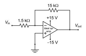
(2) (30 points) For the op amp circuit shown, find the values of  $V_{\text{out}}$  and  $i_{\text{out}}$ .
