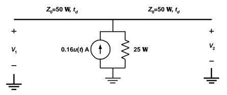
(a) (10 points) Sketch the voltage  $V_1(t)$  over the time interval  $0 \le t \le 5t_d^+$ . Provide a bounce diagram to support the  $V_1(t)$  sketch. (b) (15 points) Repeat part (a) for the following circuit. Again, please provide a bounce diagram.
