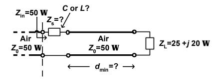
3. Matching with a single shunt lumped reactive element on a transmission line. Design the matching network shown to match a load impedance of value  $Z_L = 25+j20 \ \Omega$  to  $Z_{in} = 50 \ \Omega$  at 20 MHz. Connect the single shunt lumped reactive element as close as possible to the load. What is the type of this element, what should be its value and where should it be connected with respect to the load?
