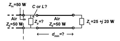
4. Matching with a single short-circuited series stub on a transmission line. Design the matching network shown to match a load impedance of value  $Z_L = 25+j20 \Omega$  to  $Z_{in} = 50 \Omega$  at 20 MHz. Connect the single short-circuited series stub as close as possible to the load. Determine the length and the location of the stub with respect to the load.
