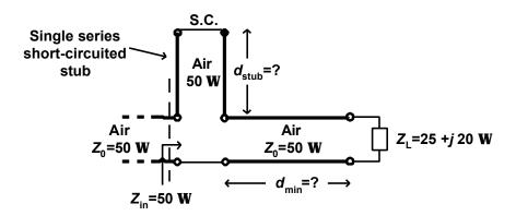
5. Matching with a single short-circuited shunt stub on a transmission line. Design the matching network shown to match a load impedance of value  $Z_L = 25+j20 \Omega$  to  $Z_{in} = 50 \Omega$  at 20 MHz. Connect the single short-circuited shunt stub as close as possible to the load. Determine the length and the location of the stub with respect to the load.
