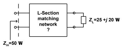
2. Matching with a single series lumped reactive element on a transmission line. Design the matching network shown to match a load impedance of value  $Z_L = 25+j20 \ \Omega$  to  $Z_{in} = 50 \ \Omega$  at 20 MHz. Connect the single series lumped reactive element as close as possible to the load. What is the type of this element, what should be its value and where should it be connected with respect to the load?
