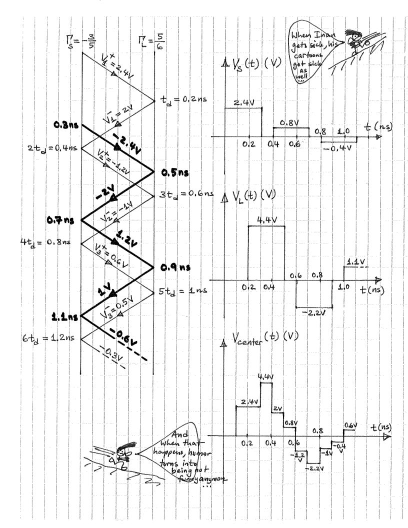
(2) (20 mins., 40 points) Lumped inductive element between two lossless transmission lines. For the transmission line circuit shown, <u>find</u> and <u>sketch</u> the source-end and load-end voltages as a function of time. Show your work and provide all the appropriate values on your sketches.
