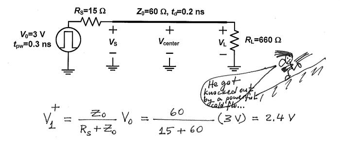
$$\frac{7}{L} = \frac{R_L - Z_0}{R_L + Z_0} = \frac{660 - 60}{660 + 60} = \frac{600}{720} = \frac{5}{6}$$
