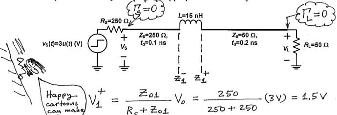
Since the inductor will at first act like an open circuit, we have  $V_1(\overline{z_1}, t_{d1}) = V_1 = 1.5 \text{V}$ . However, when the inductor reaches steady state, it acts like a short circuit and as a result, we have  $V_1(\overline{z_1}, \infty) = \frac{Z_{02} - Z_{01}}{Z_{02} + Z_{01}} V_1 = \frac{50 - 250}{50 + 250} (1.5 \text{V})$  = -1 V. The time constant of the circuit can be found as
