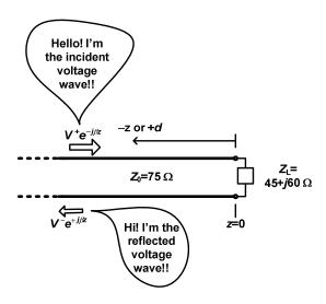
(a) (10 points) Calculate the load reflection coefficient,  $\Gamma_L$ . (Provide your answer in polar form.) Show your work!
