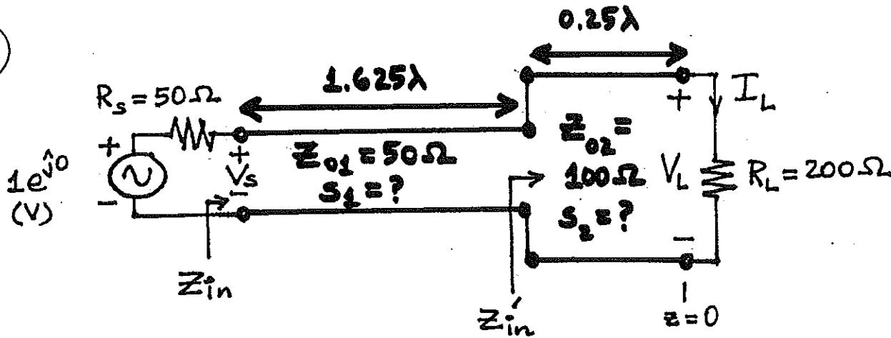
$$(a) \Gamma_L = \frac{R_L - Z_{02}}{R_L + Z_{02}} = \frac{200 - 100}{200 + 100} = \frac{1}{3}$$
