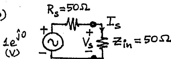
$$V_s = \frac{Z_{in}}{R_s + Z_{in}} (1e^{j0}) = 0.5V, I_s = V_s/Z_{in} = 10mA$$
