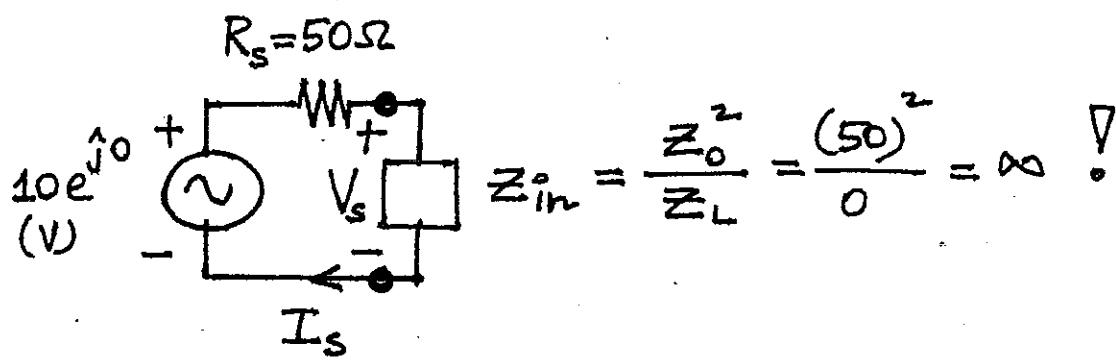
$$\therefore I_s = 0 \quad \& \quad V_s = 10e^{j0} \text{ (V)}$$
