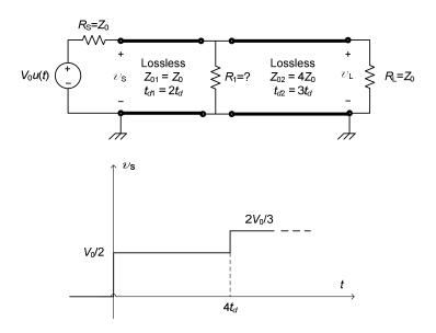
(a) (15 points) Determine the value of the lumped resistor  $R_1$  in terms of the characteristic impedance  $Z_0$ .
