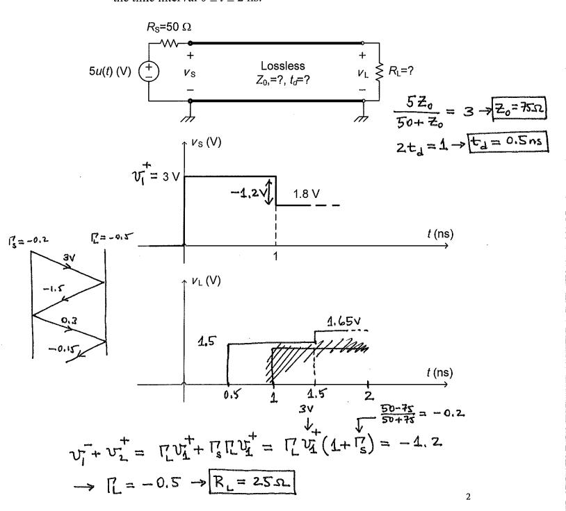
(2) (15 mins., 35 points) Multiple transmission lines. For the three transmission-line circuit shown, the switch closes at t = 0. Assuming all the lines to be uncharged before t = 0, sketch voltages  $\mathbf{v}_S$ ,  $\mathbf{v}_{L1}$  and  $\mathbf{v}_{L2}$  between t = 0 to 10 ns. Use bounce diagram. Provide all the pertinent
