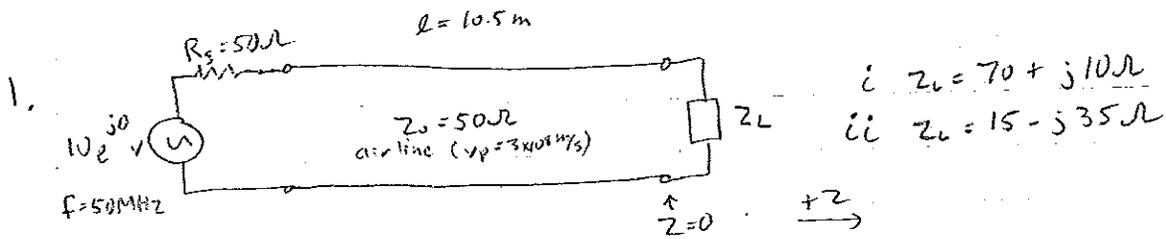
$$\lambda = \frac{v_p}{f} = \frac{3 \times 10^8 \text{ m/s}}{50 \text{ MHz}}$$
