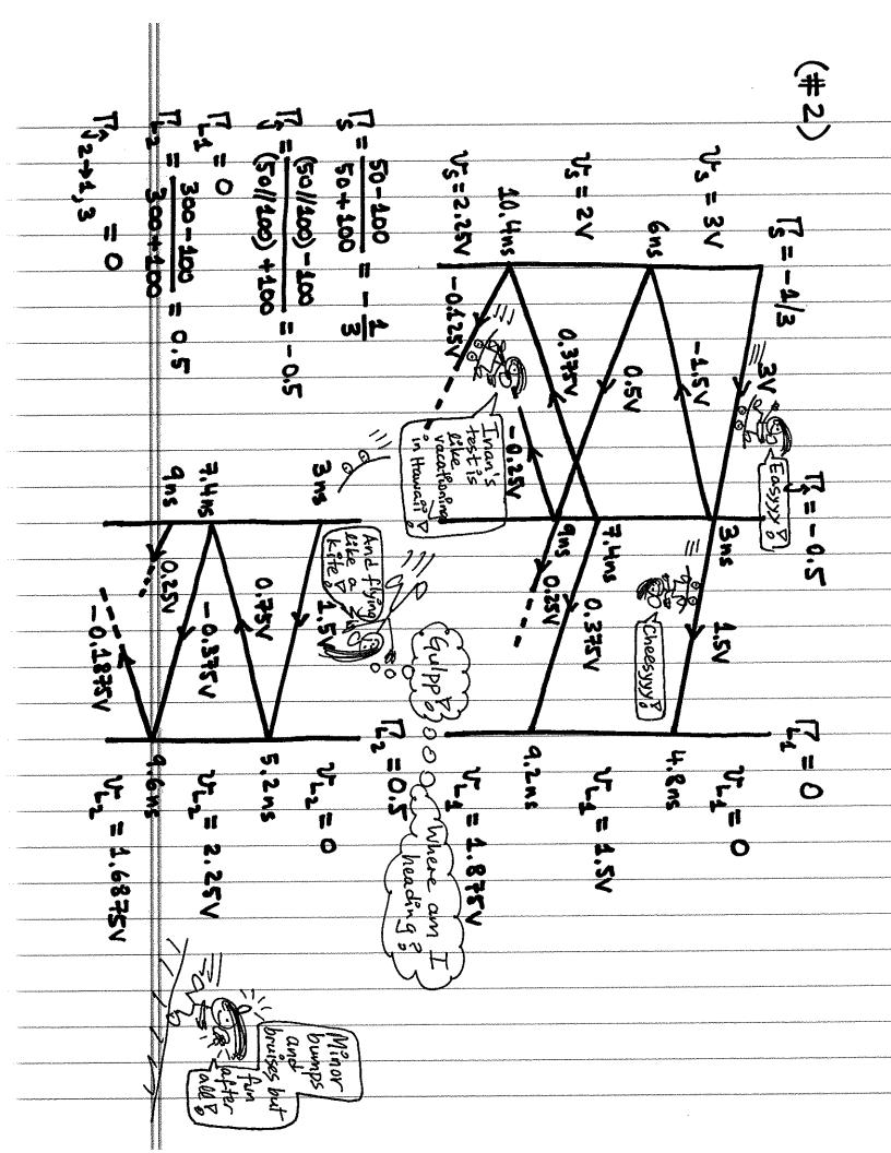
(3) (15 mins., 35 points) Reactive element at the junction. In the transmission-line circuit shown, find the complete mathematical expressions and sketch both the source-end voltage  $v_S$  and the load-end voltage  $v_S$  as a function of time. Sketch the two waveforms separately.
