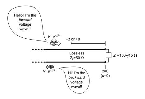
(a) (10 points) Calculate the load reflection coefficient,  $\Gamma_L$ . (Provide your answer in polar form.) Show your work!
