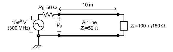
(a) (10 points) Calculate the load reflection coefficient  $\Gamma_L$ . (Provide your answer in polar form.) Show your work!
