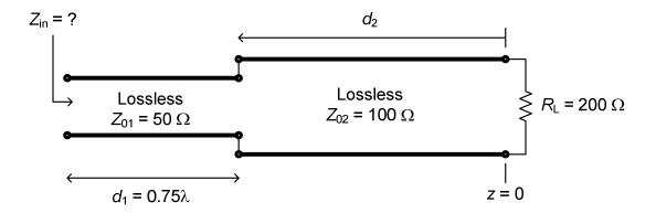
(6) Source- and load-end voltages. For the transmission line shown, assuming sinusoidal steady state, calculate the source-end and load-end voltages  $V_S$  and  $V_L$  in phasor form.
