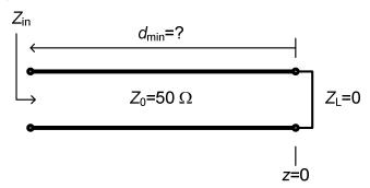
(4) Open- and short-circuit impedance measurements. If the open- and short-circuit terminated input impedances of a lossless transmission line with characteristic impedance  $Z_0$ , length d and phase velocity  $v_p = 2c/3$  are measured at 5 GHz to be  $Z_{oc} = -j500 \Omega$  and  $Z_{sc} = j20 \Omega$  respectively, calculate  $Z_0$  and the length d of this line. (Note that  $c = 3 \times 10^8$  m/s.)
