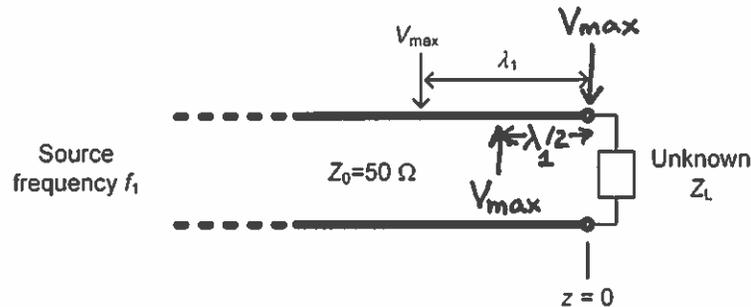
$$S = \frac{1 + |\Gamma_L|}{1 - |\Gamma_L|} \rightarrow |\Gamma_L| = \frac{S - 1}{S + 1} = \frac{5 - 1}{5 + 1} = \frac{2}{3}$$
