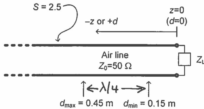
$$(a) \quad \frac{\lambda_{\text{air}}}{4} = 0.45 - 0.15 = 0.3 \text{ m} \rightarrow \lambda_{\text{air}} = 1.2 \text{ m}$$
