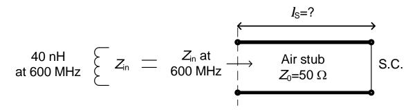
(b) Design a 40 nH inductor using an open-circuit terminated 50  $\Omega$  air stub at 600 MHz.
