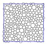
Instability in 256 disks — DEM simulation Biaxial compression
