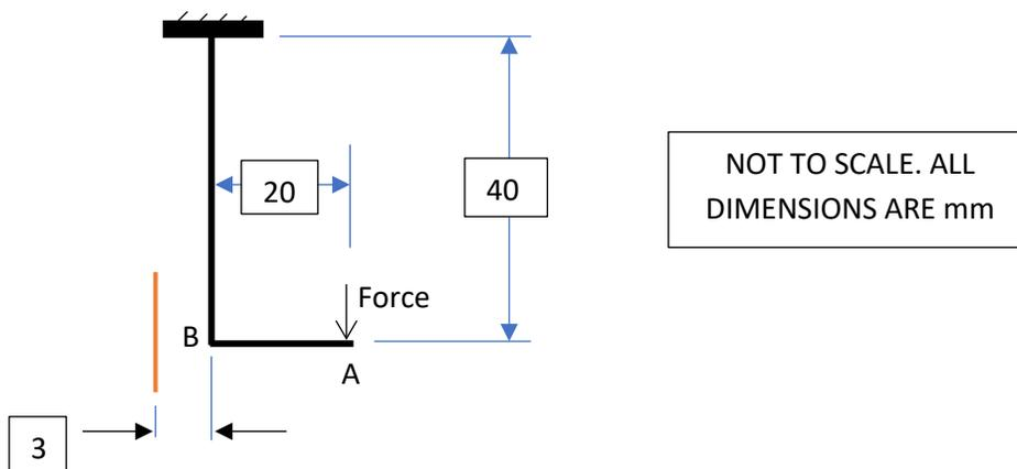
2. Script for the Echidna beam is provided on the course page – run it with at least two different SMRTSIZE sizes. Analyze the stress in the x-direction. Note that the beam will look much longer than the workbook beam – the workbook beam is not to scale.
