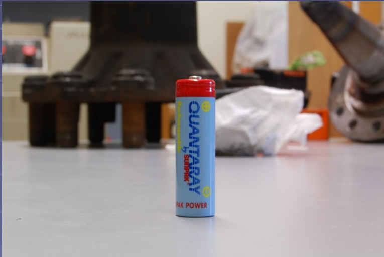
Small aperture (F/22) Long depth of field
