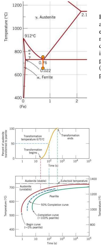
Phase diagrams assume phases are at equilibrium. Time is not relevant to phase diagrams. However, it does take time for phase transformation (to change from one phase to another).
