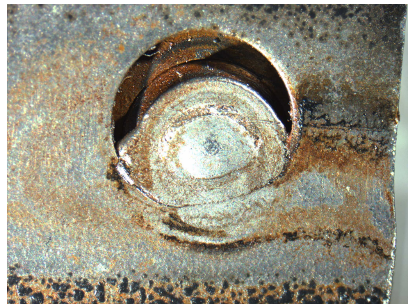
Figure 4 – close up of failed weld on tab “E” (see figure 3). The “rust” (red) likely developed sometime after testing.
