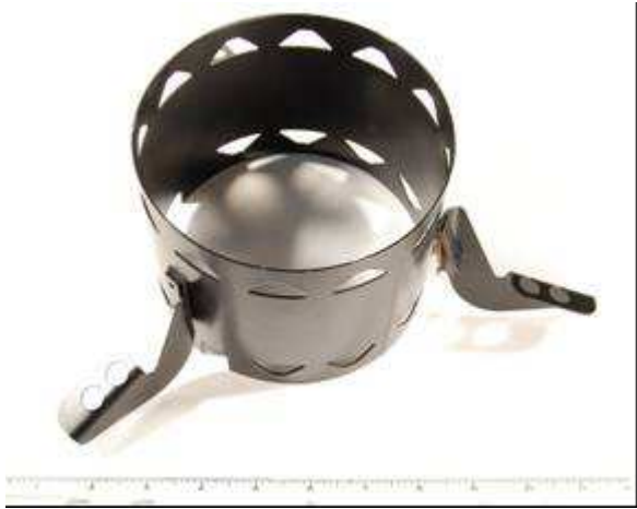
Figure 1 – band with legs (leg on right has been “chisel” tested).
