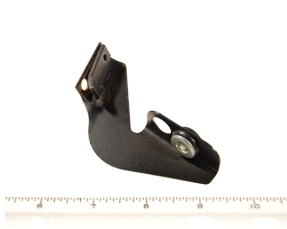
Figure 2 – leg that has been chisel tested.
