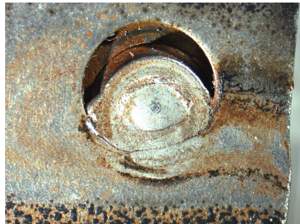
Figure 4 – close up of failed weld on tab “E” (see figure 3). The “rust” (red) developed sometime after testing.
