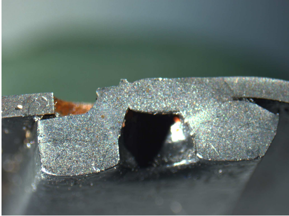
Figure 5 – close up of cross-section through failed weld, tab Sample “E” in Figure 3.
