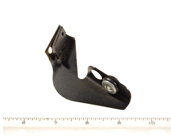
Figure 2 – leg that has been chisel tested.
