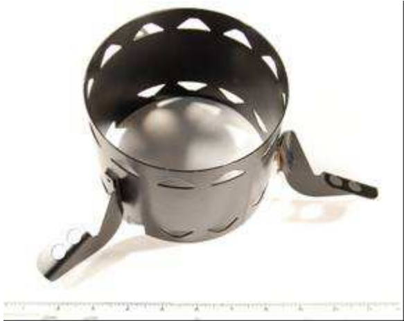
Figure 1 – band with legs (leg on right has been “chisel” tested).
