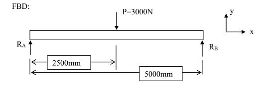
$$\begin{split} R_A &= 0.5*P = 1500 \text{N} \text{ (due to symmetry, } R_A = R_B \text{ and } R_A + R_B = 3000 \text{N} \text{)} \\ \sigma &= My/I \\ \text{M} = \text{moment at load application} = R_A*L_A = 1500 \text{N}*2500 \text{mm} = 3,750,000 \text{ N-mm} \\ y &= \frac{1}{2}*\text{Dia} \text{ (distance from neutral axis to top/bottom of beam)} \\ I &= \pi D^4/64 \text{ (back cover of Shigley's Machine Design text)} \end{split}$$
