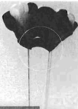
Self-help in a ram-air parachute—air speed both opens the parachute and holds it closed.
