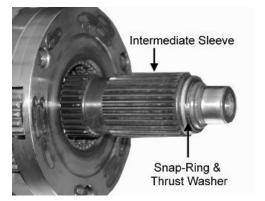
External clip – meant for retaining objects such as bearings on a shaft. Note that there are grooves cut into shafts for the retaining rings. The grooves are stress concentrations and the shaft designer must consider that (keep the nominal stresses low). Retaining rings cannot hold much thrust loads – but enough to keep bearings and such from "walking" (moving with minimal "push or
