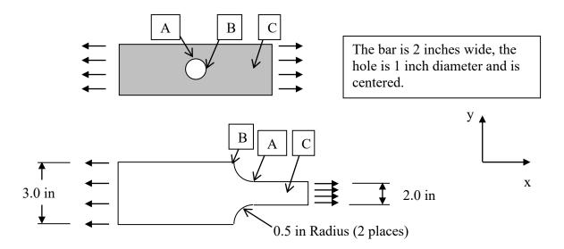
**DESIGN PROBLEM.** Educational Purpose: The second problem shows that stress concentration charts can be used for parametric design analysis (the parameter being the hole diameter). FEA is not always a good design tool – it is a good analysis tool. The charts can effectively be used for design. Please see course web page for general requirements associated with homework using Excel. Why Excel? Many employers have commented that they want engineers who are competent with Excel.
