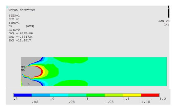
The nominal stress (F/A) is 1 psi. At a distance of about 1 plate width, the stress becomes uniform to within about 5% (all colors are with the 0.95psi to 1.05psi stress range). Note, this model uses PLANE182 (2D) elements. The plate is 1" wide (by 1" thick) and 5 inches long – the right side is constrained in the y-direction to create symmetry.
